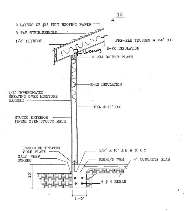
TYPICAL WALL SECTION AND FOOTING DETAIL
